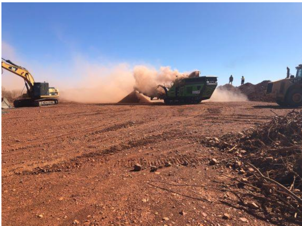
Impact crusher producing gravel
